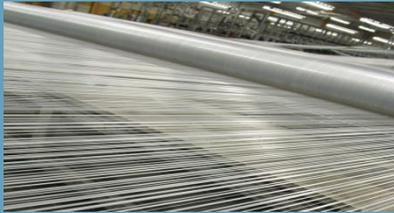
Yarn performance in a beaming process can be affected by the entanglement strength in the yarn. One important characteristic of the entangled yarn relates to the strength of the individual entanglements. The entanglements serve to provide the yarn bundle with cohesiveness so that the downstream conversion of the yarn into a fabric will occur with a minimum of defects.
